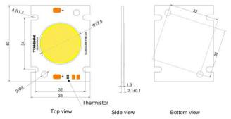
LED COB 250W 3200K LED PFE-200 3000K Profile Spot (TX-3850S200C28F12-03H95)
