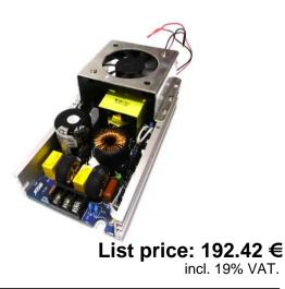
Platine (Power supply) V1:28V V2:12V /600W LED TMH-X19 (NW152B-W600U28&12)
