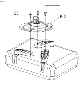
Setting B-2 subassembly on projector unit by part 23 as per drawing.
