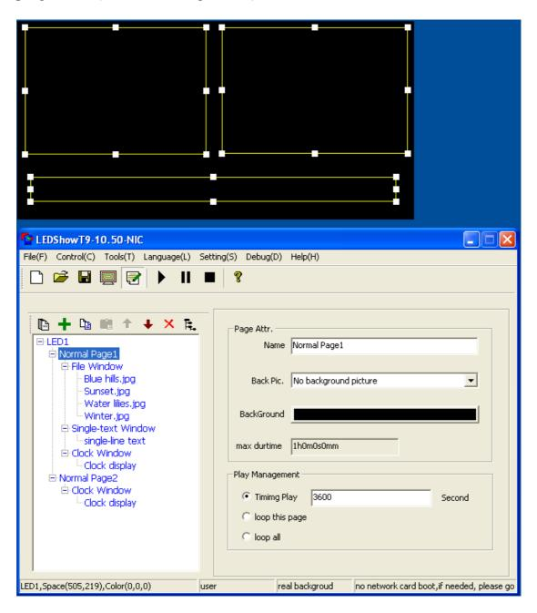
Figure 3-2 Schematic diagram of Programme Composition
