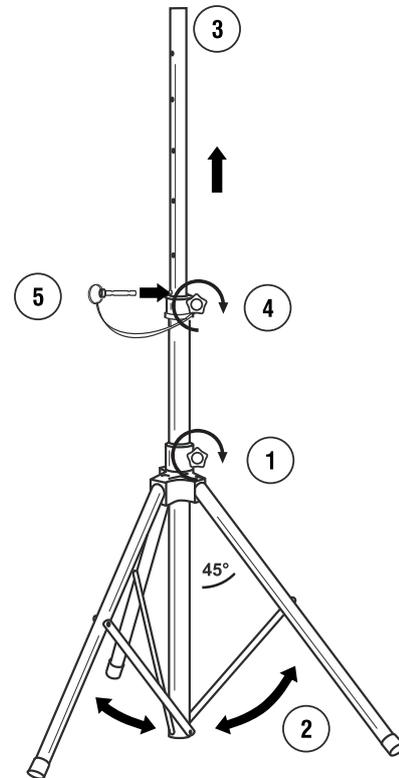
**Pull out the legs** – Loosen the safety screw (1) of the legs. Pull out the legs (2). Lock this position with the safety screw.
