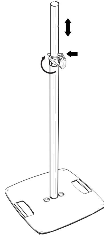
**Setup** - Screw the stand tube into the thread in the base plate.
