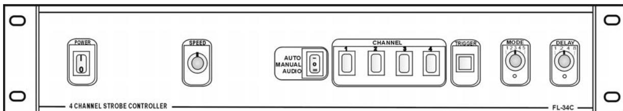
**Power:** to switch the unit on and off.
