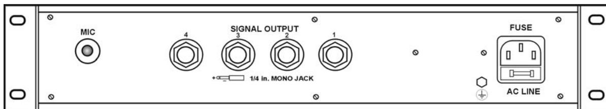
Use the Mono Jack (1/4") for connecting your strobe(s) (up to 5 units). Use a one-cord lead with screen (1 x 0,22) as connection cable.
