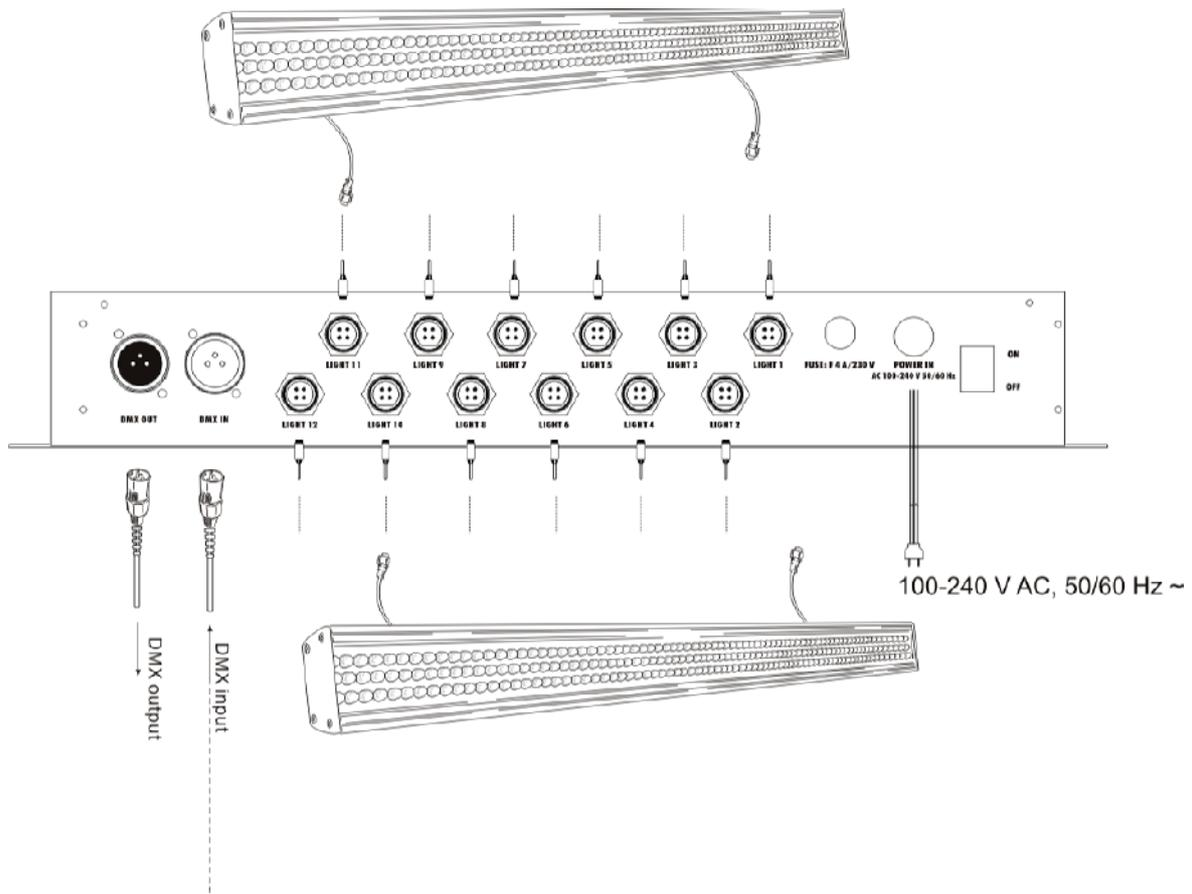
Connect the luminaire to one of the 4-pin connection cables of the controller. A maximum of 12 LED Bar 12V RGB 100cm devices can be connected to the LED PSI-1 DMX Controller.
