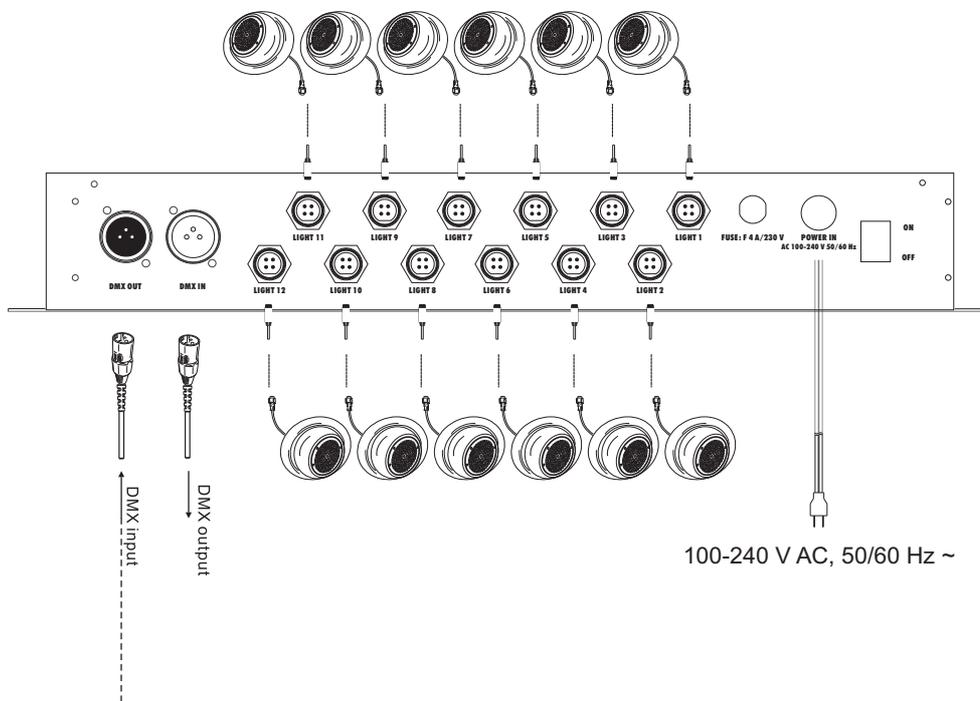
Connect the luminaire to one of the 4-pin connection cables of the controller.
