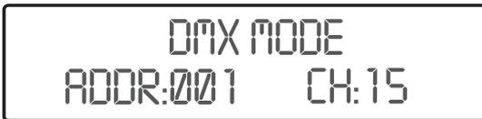
Press the MODE button until the display shows DMX MODE.
