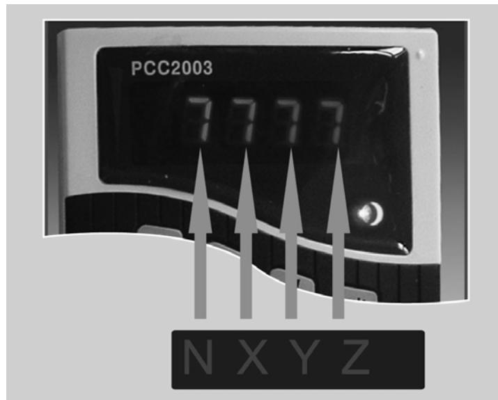
**N, X, Y, Z** correspond to the four numbers on the display with „channels“ from 0-9.
