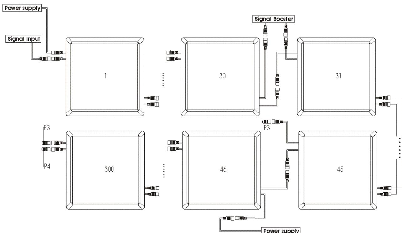
P3 = 2-pin power supply lead socket
