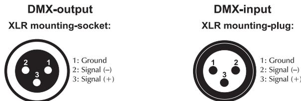
If you are using controllers with this occupation, you can connect the DMX-output of the controller directly with the DMX-input of the first fixture in the DMX-chain. If you wish to connect DMX-controllers with other XLR-outputs, you need to use adapter-cables.
