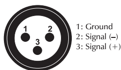
DMX-input XLR mounting-plug:
