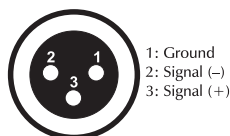
DMX-output XLR mounting-socket:
