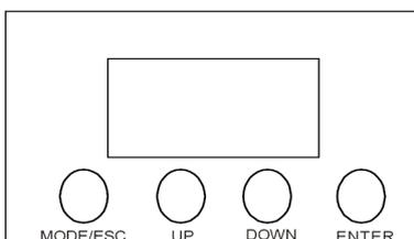
The control board offers several features, i.e. setting the DMX starting address, running a preset program or selecting a DMX channel mode.
