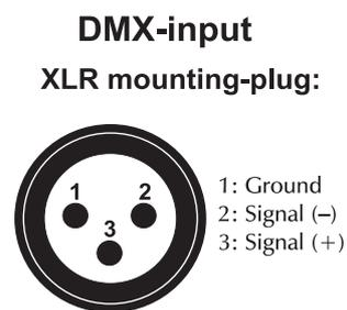
If you are using controllers with this occupation, you can connect the DMX-output of the controller directly with the DMX-input of the first fixture in the DMX-chain. If you wish to connect DMX-controllers with other XLR-outputs, you need to use adapter-cables.
