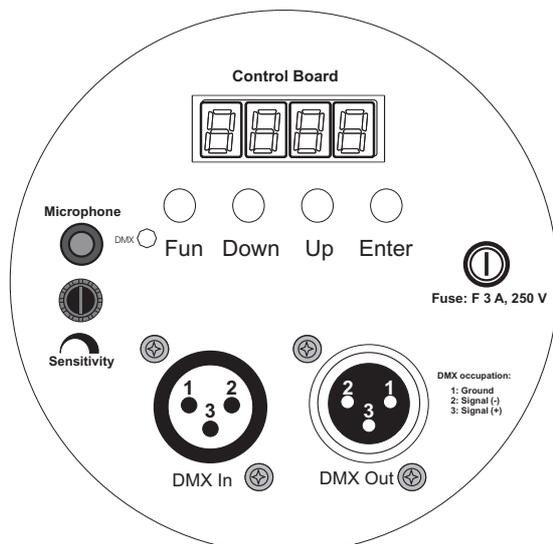
The Control Board offers several features: you can e. g. simply set the starting address.
