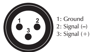
DMX-input XLR mounting-plug:
