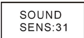
With this point of the menu, you can activate the slave mode. Via buttons UP/DOWN, you can define the input level (SENS) between 0 and 31.
