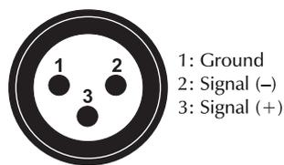
If you are using controllers with this occupation, you can connect the DMX output of the controller directly with the DMX input of the first device in the DMX chain. If you wish to connect DMX controllers with other XLR outputs, you need to use adapter cables.
