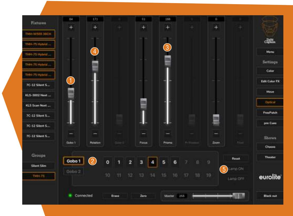
This page contains the various optical functions of spotlights. Gobos and their rotation can be accessed via the sliders ①, but the gobos can also be accessed via the direct selection buttons ② at the bottom. At “Prisma” ③, it depends on the fixture whether the rotation is already on this slider or on the “Rotation” slider ④. “Reset”, “Lamp On” and “Lamp Off” ⑤ must receive the command for about 3 seconds with most fixtures until triggered.
