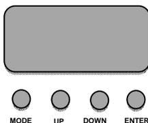
Browse through the menu by pressing Mode. Press Enter in order to select the desired menu. You can change the selection by pressing Up or Down. Press Enter in order to confirm. You can leave every mode by pressing Mode. The functions provided are listed in the following sections.
