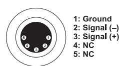
DMX-output XLR mounting-socket:
