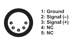
DMX-input XLR mounting-plug:
