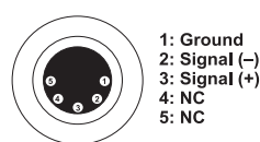
DMX-output XLR mounting-socket:
