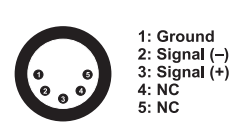
DMX-input XLR mounting-plug:
