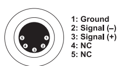
DMX-output XLR mounting-socket:
