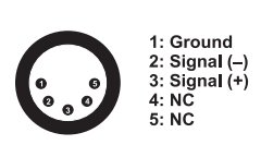
DMX-input XLR mounting-plug:
