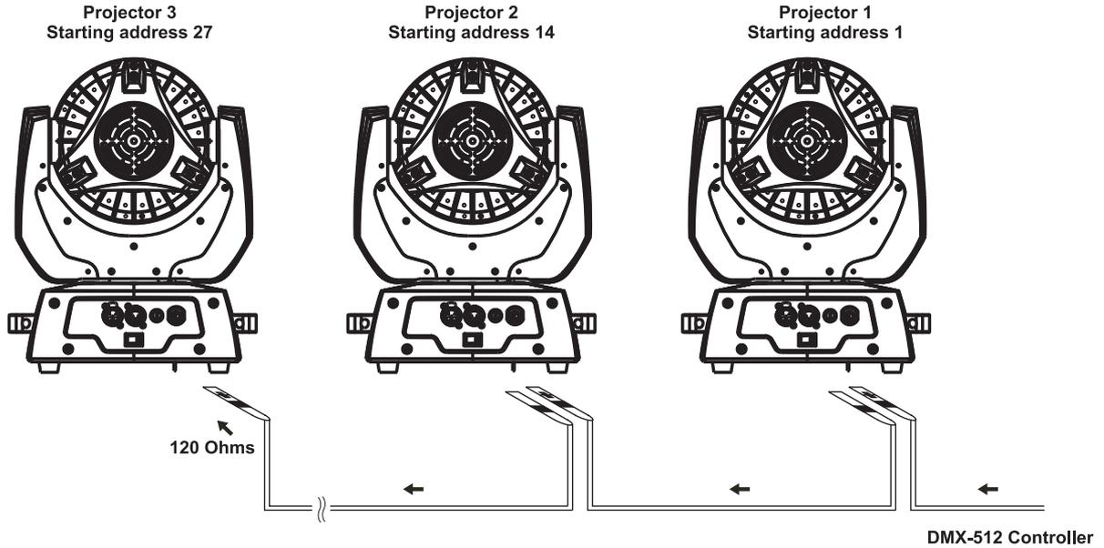
**! The wires must not come into contact with each other, otherwise the fixtures will not work at all, or will not work properly. !**
