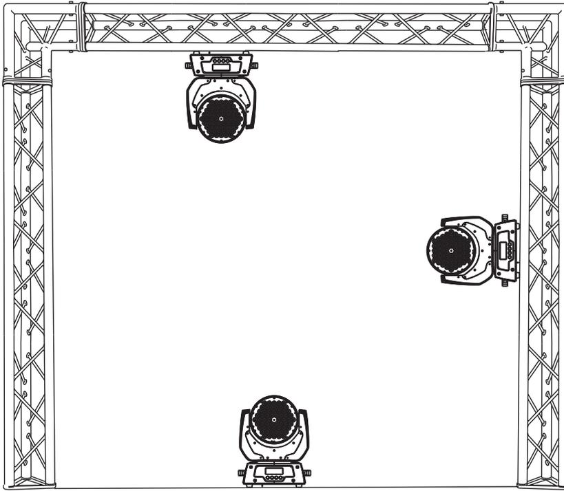
The Moving-Head can be placed directly on the stage floor or rigged in any orientation on a truss without altering its operation characteristics (see the drawing).
