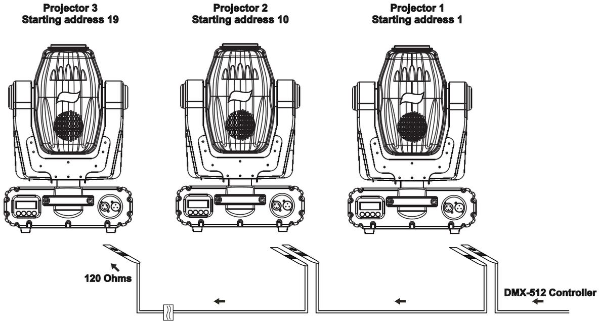
**! The wires must not come into contact with each other, otherwise the fixtures will not work at all, or will not work properly. !**
