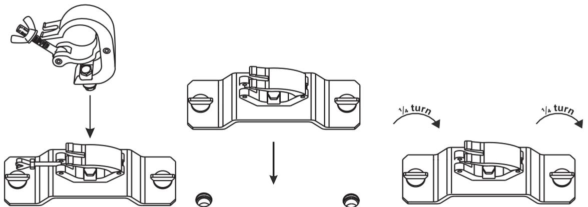
Screw one clamp each via a M12 screw and nut onto the Omega-holders.
