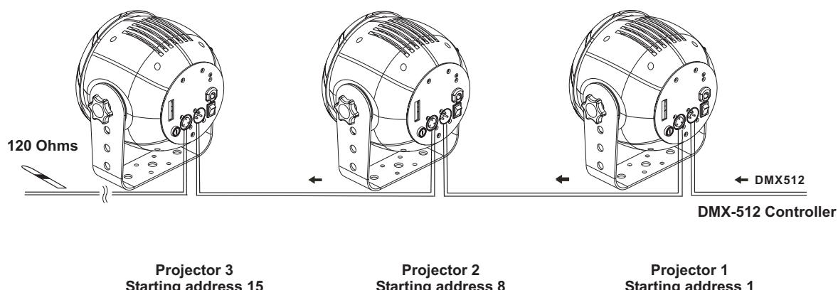
**The wires must not come into contact with each other, otherwise the fixtures will not work at all, or will not work properly.**
