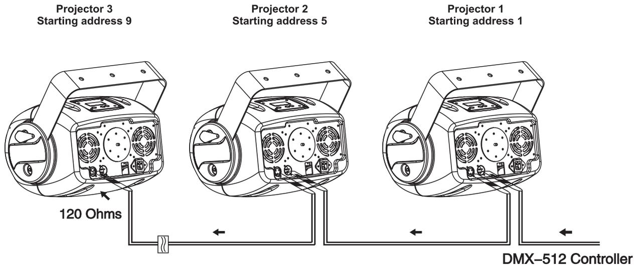
**! The wires must not come into contact with each other, otherwise the fixtures will not work at all, or will not work properly. !**
