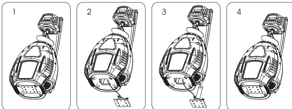
**Step 1:** Unscrew the fixation screws X, Y, Z of the lamp system and carefully remove it from the housing.
