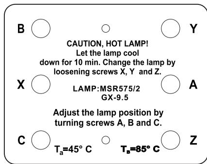
The lampholder is aligned at the factory. Due to differences between lamps, fine adjustment may improve light performance.
