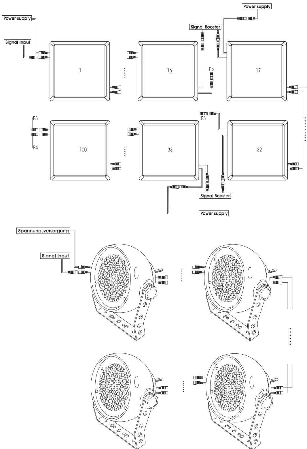
**Attention:** After every 16 PPP-60 panels, 16 WP-60 LED-wall panels, 16 PS-144 spots or 16 CPS-144 spots the fixtures must have a renewed connection with the power mains.
