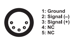
DMX-input XLR mounting-plug:
