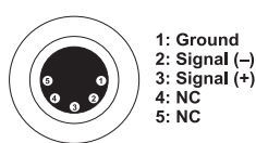
DMX-output XLR mounting-socket:
