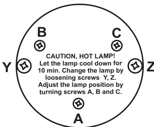
The lampholder is aligned at the factory. Due to differences between lamps, fine adjustment may improve light performance.
