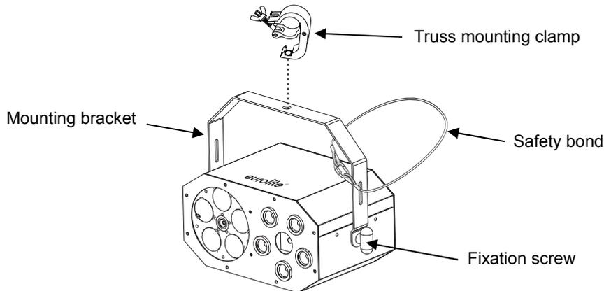
The device may be placed on the floor or fastened to a truss or similar rigging structure. The device must never be fixed swinging freely in the room.
