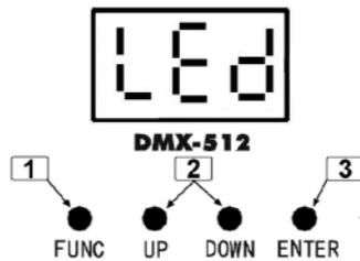
In the COLOR CHOICE setting, the LED COLOR that you are going to choose is flashing. Press UP or DOWN to change the LED color, you will have 10 different LED color mode. Their DISPLAY and EFFECT are listed below:
