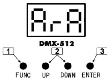
In the MODE OPTION setting, the stand alone laser show that you are going to choose is flashing. Press UP or DOWN to change stand alone laser show, you will have 8 different stand alone preprogrammed laser show. Their DISPLAY and EFFECT are listed below:
