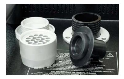
After use or before moving, remove the cap and fix it on the left and use rubber cork as stopper for the fluid tank as below picture shows.
