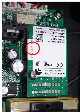
**Step 7. Install the W-DMX onto the main PCB and then screw the screw tightly. The installation of W-DMX antenna and W-DMX board is completed.**
