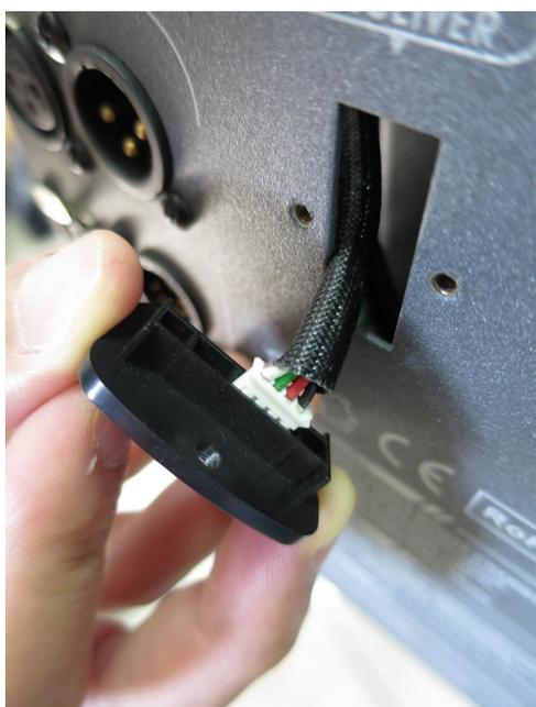
Step 3: Connect the terminal to W-1 Wireless Signal Receiver.
