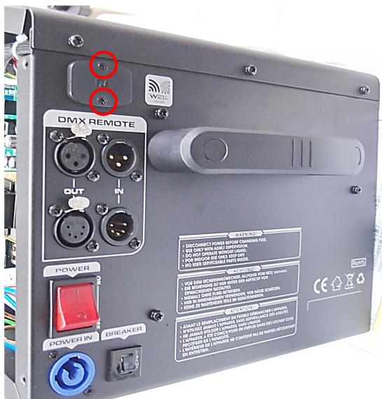
**Step 3. Remove the cover on the control panel.**
