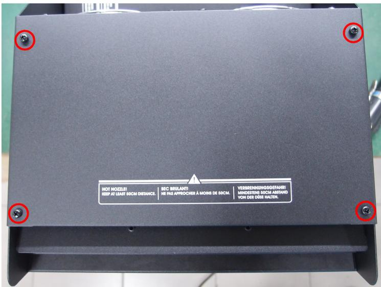
**Step 1. Remove the screws on the top of F-1.**
