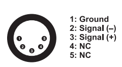
DMX-input XLR mounting-plug:
