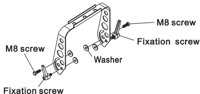
Screw the mounting bracket to the machine using the included set of screws. Place the washers on the inside of the bracket and adjust the desired inclination angle. Tighten the fixation screws.
