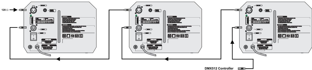
Use a DMX cable and 3-pin or 5-pin XLR plugs and connectors in order to connect the controller with the fixture or one fixture with another. If you wish to connect DMX controllers with other XLR outputs, you need to use adapter cables.
