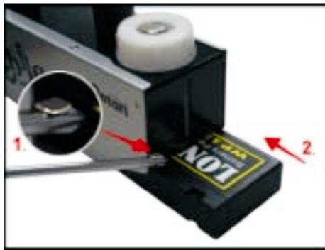
1. Lift-up the plate before inserting the battery.
