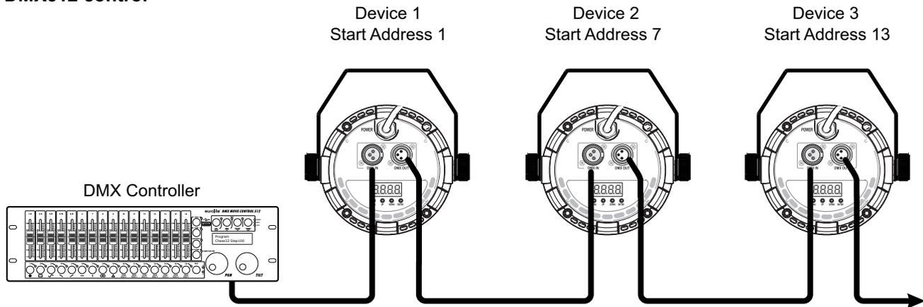
A DMX512 data link is required in order to control the device via DMX. The device provides 3-pin XLR connectors for DMX connection.
