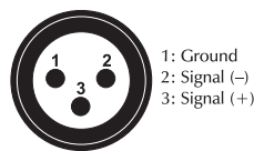
DMX-input XLR mounting-plug:
