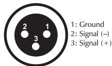
DMX-output XLR mounting-socket:
