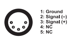
DMX-input XLR mounting-plug:
