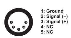
DMX-input XLR mounting-plug:
