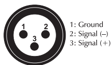
DMX-input XLR mounting-plug:
