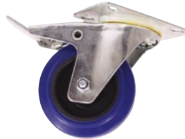
No. 3000400B ROADINGER Swivel castor 100mm with brake • Double-action brake (wheel and swivel) • Housing made of steel, zinc-plated • Blue elastic tyre • Roller-race hub bearing • Height: 128 mm
