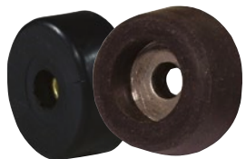
No. 30001200 .....large, steel-reinforced No. 30001202 ..... 25 x 25 mm No. 3000130A .....small, with steel ring ROADINGER Rubber foot • With steel disk insert • Diameter: 38 mm • Height: 20 mm • Weight: approx. 30 g • Mounting hole: d= 5.5 mm
