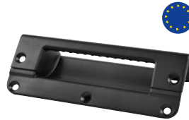
No. 30000830 ROADINGER Insert dish handle, black plastic • Cut-out 50 x 95 mm • Weight approx. 40 g • Mounting holes: d=5.0 mm
