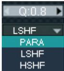
Under “**Type**“ three filter types can be selected: PARA (default setting), LSHF (Low Shelving Filter = low frequency filter with shelving characteristic) and HSHF (High Shelving Filter = high frequency filter with shelving characteristic). The quality factor (Q) and thus the filter's slope can be adjusted in the “**Q Value**“ field.
