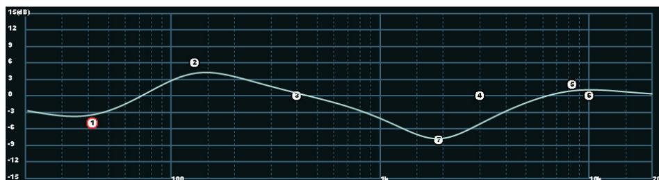
The parameters can also be adjusted graphically via the frequency curve. A graphical reference point (white circle with red marking) next to the curve is shown. By moving the point horizontally with the mouse, the frequency can be changed; by moving the point vertically the gain can be adjusted.
