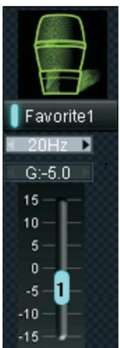
Enter the filter frequency in the “FC” field or click the arrows. For gain adjustment, use the “Gain” field or the slider.
