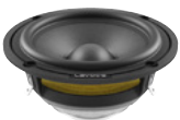
No. 12602918 LAVOCE FAN030.71 3" Fullrange Neodymium Magnet Aluminium Basket Driver 30 W AES, 8 ohms, 89.5 dB, 120-21000 Hz
