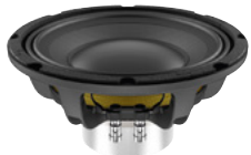
No. 12602616 LAVOCE WAN103.00 10" Woofer Neodymium Magnet Aluminium Basket Driver 450 W AES, 8 ohms, 93 dB, 50-1500 Hz
