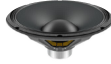
No. 12602620 LAVOCE SSN153.00 15" Subwoofer Neodymium Magnet Steel Basket Driver 400 W AES, 8 ohms, 98 dB, 50-3000 Hz
