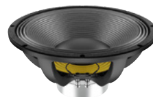
No. 12602624 LAVOCE WAN154.00 15" Subwoofer Neodymium Magnet Aluminium Basket Driver 1500 W AES, 8 ohms, 95.5 dB, 40-1000 Hz
